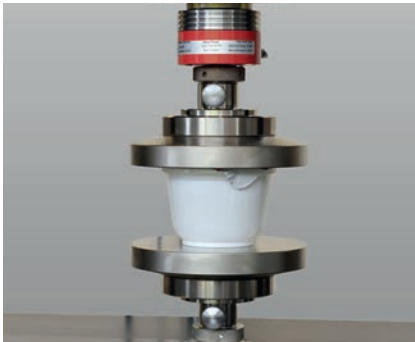
Fig. 1: Determining stackability of hollow packagings and drinks crates
