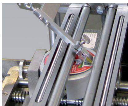
Fig. 2: Testing the sealed seam on a yoghurt pot. The peel angle remains constant.
