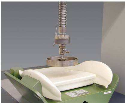
Fig. 3: Indentation hardness of molded foam parts (DIN 53579-1)
