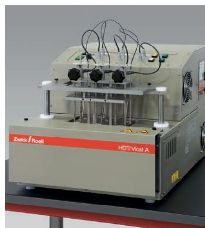
Fig. 2: Allrounders HDT/Vicat 3-300A and 6-300A are fitted with a hoist, enabling the entire test to run automatically. They are equipped with a bath to accommodate three or six measuring stations.
