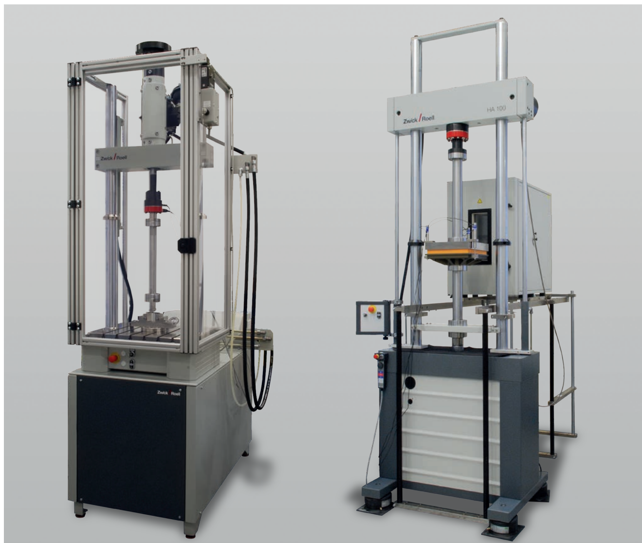
Fig. 1: Servo-hydraulic testing machines for rapid cyclic loading
