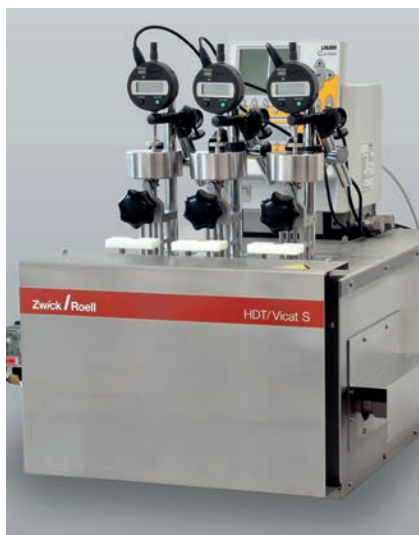
Fig. 2: HDT/Vicat 3-300 S basic instrument: measurements up to 300 °C, 1 to 3 stations
