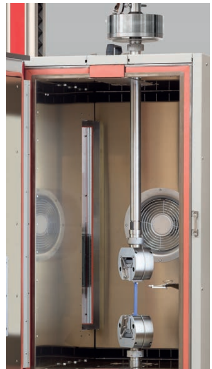
Fig. 6: The Modular BoW gripping system allows easy change of configuration
