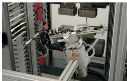
Fig. 1: Automated feeding of up to 20 rigid tensile specimens 'roboTest A'.
