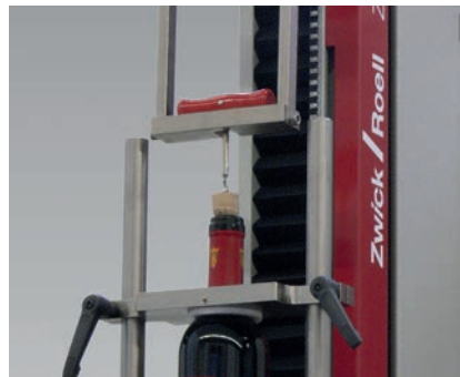
Fig. 6: Extraction tests on bottle corks
