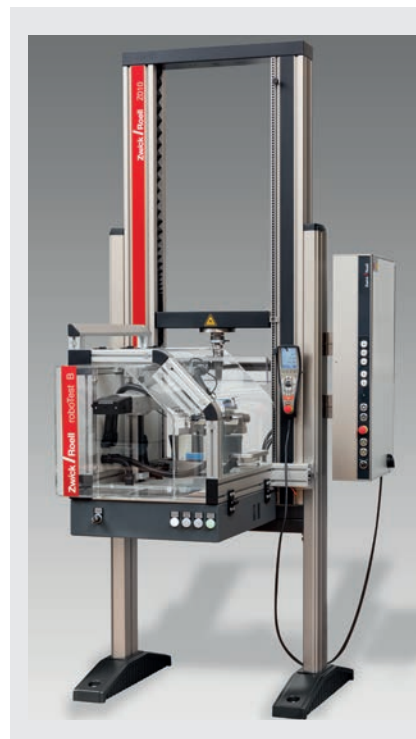
Fig. 2: 'roboTest B' - easy changeover between tensile and flexural testing. Automatic specimen feed from magazines holding up to 20 specimens
