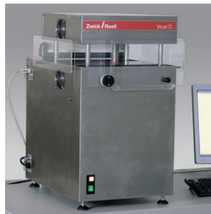
Fig. 3: The Vicat Dry's oil-free measuring principle ensures clean working conditions
