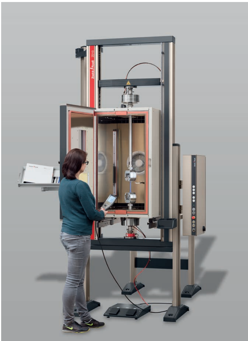
Fig. 1: AllroundLine testing machine with temperature chamber in testing position. Extension measurement is via a side port.
