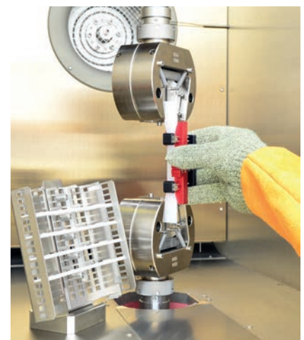
Fig. 3: Optional magazine for preconditioning of specimen.
