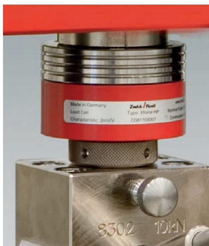
Fig. 1: Load cells for the most demanding quality requirements. Left: a load cell from the Xforce range. Center: Xforce HP design uses the ring-torsion measurement principle.
