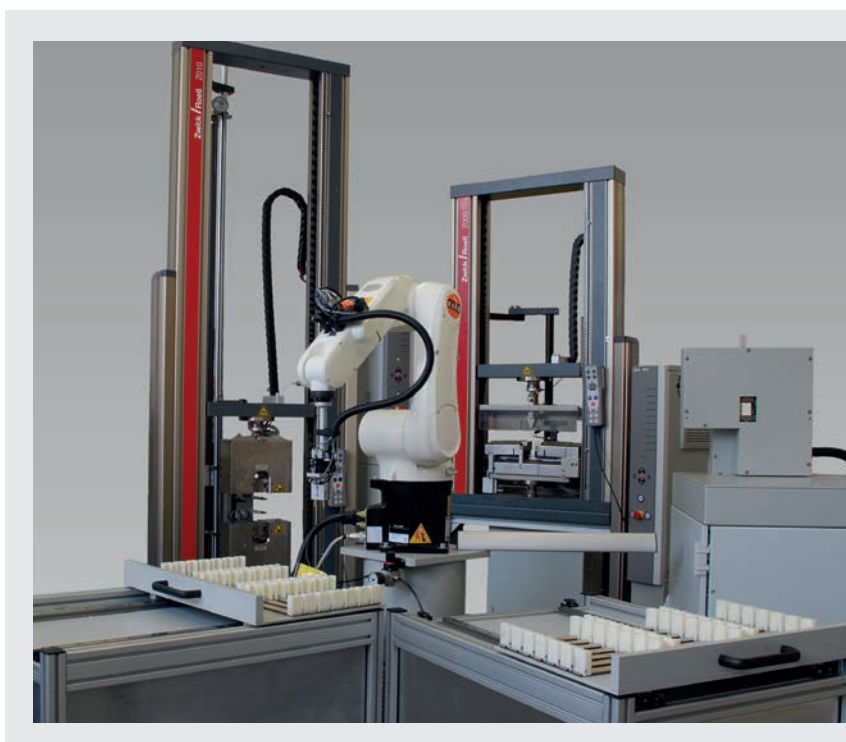
Fig. 2: 'roboTest R' - specimen feeding system incorporates multiple testing equipment, e.g. for tensile and flexure tests, impact and hardness tests. Large specimen magazine and tests in temperature chambers are functions of this system.
