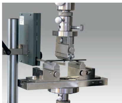
Fig. 3: Flexure transducer for 3 and 4-point measurement
