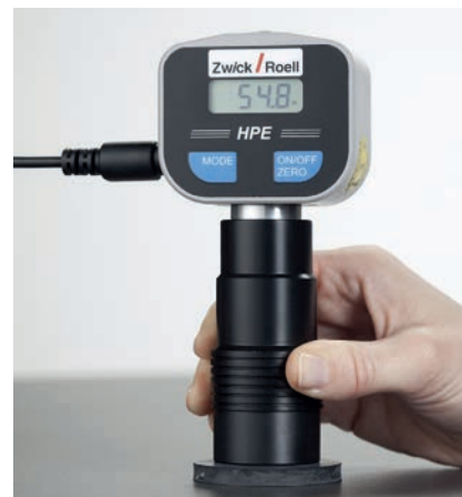
Fig. 4: Digital Shore hardness tester with integral electronics unit
