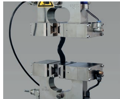
Fig. 3: Tear-growth test on an angle-type specimen to ISO 34-1
