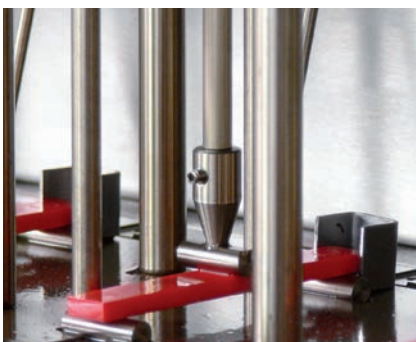
Fig. 3: HDT test to ISO 75-2: specimen are heated at a constant rate in liquid transfer medium
