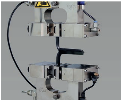
Fig. 2: Tear test on a trouser-type specimen as per ISO 34-1
