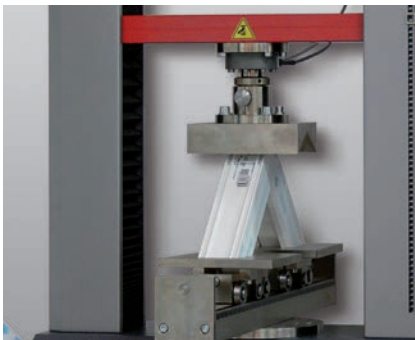
Fig. 3: Corner strength of a window frame
