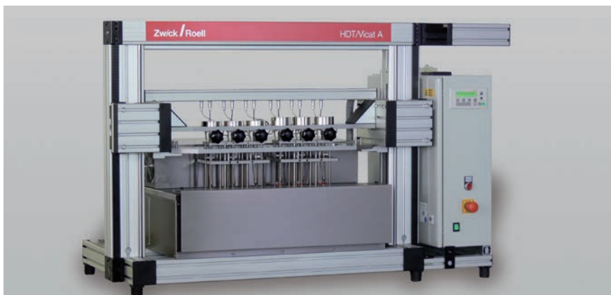
Fig. 1: The HDT/Vicat 3-300 A and 6-300A with integrated heat exchanger and three or six measuring stations.
