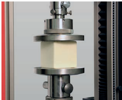
Fig. 3: Compression test to ISO 844, with and without direct travel measurement
