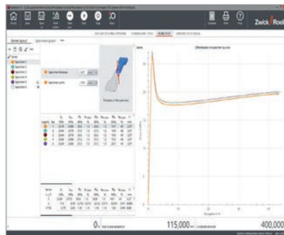
Fig. 1: Tensile test to ISO 527-2 with tensile modulus determination (moulding material characterization)
