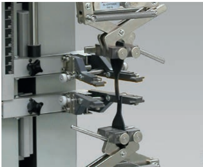
Fig. 1: Tensile test to ISO 37, ASTM D 412
