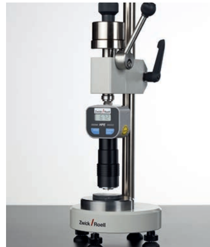
Fig. 5: Digital Shore hardness tester with test stand
