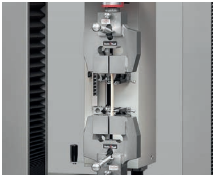
Fig. 2: Tensile test, e.g. to ASTM D 638. (quality control)
