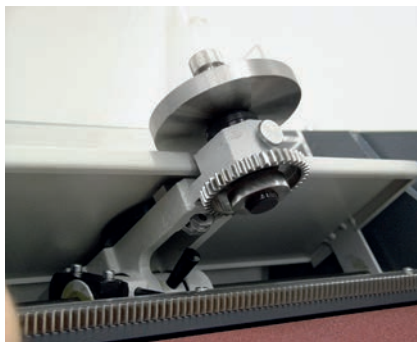
Fig. 1: Abrasion resistance, ISO 4649
