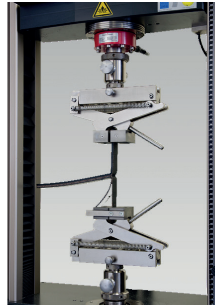
Fig. 2. Adhesion test to determine the adhesive strength between constitutive elements
